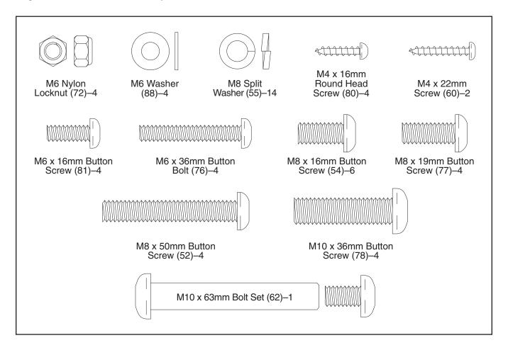
1. Attach the Left Front Stabilizer (15) to the left side of the Frame (1) with three M8 x 16mm Button Screws (54) and three M8 Split Washers (55).
